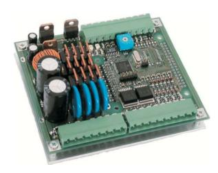
The device HS2/F1/ECO (called HS2 in this document) is used to control H+L punching systems ECO All specific processes of ECO are defined in the firmware of HS2. Thus, the user control (CNC / PLC) does not need to implement these processes.
